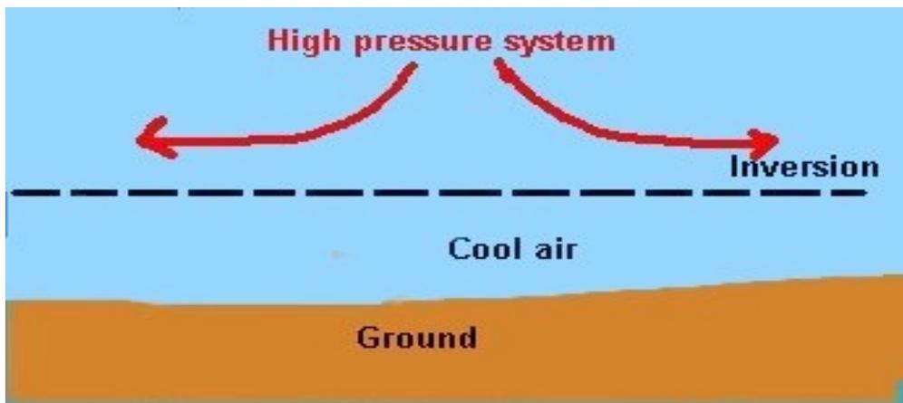
**Radiative inversion** forms when heat is rapidly lost from the surface by thermal radiation.
