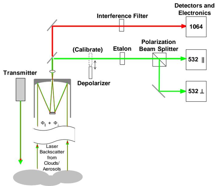
**Figure 23.4** Functional block diagram of CALIOP (from CALIPSO ATBD).
