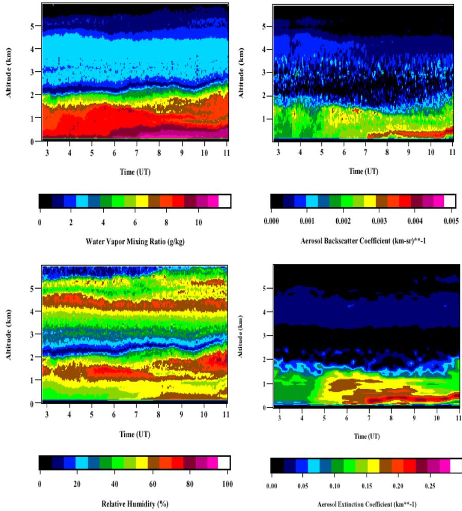
**Figure 23.1** Examples of retrievals using the Raman lidar.
