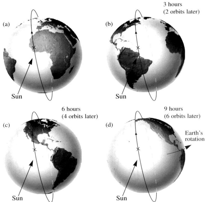
**Figure 1.7** Oblique orbiting (near-polar orbiting) satellites: Sun-synchronous orbits (each 3 hours)
