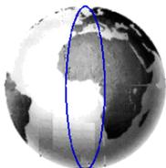
Polar orbiting satellites, whose orbits are in the plane of the Earth's polar axis
