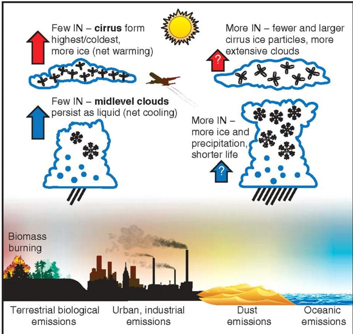
**Figure 2.7** Schematic diagram of the effect of ice nuclei from various possible aerosol sources on midlevel precipitating clouds and cirrus ice clouds. The likely but uncertain change in the magnitude of the general cooling impact (blue arrows) of midlevel clouds and warming impact (red arrows) of high cirrus clouds in response to increases in the relative number concentrations of IN is indicated (From DeMott et al., PNAS, 2010;107:11217-11222)
