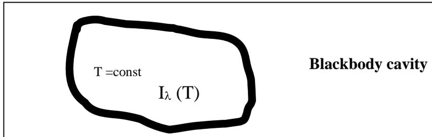
**NOTE:** A blackbody cavity is an important element in the design of radiometers. Cavities are used to provide a well-defined source for calibration of radiometers. Another use of a cavity is to measure the radiation that flows into the cavity (e.g., to measure the radiation of sun).
