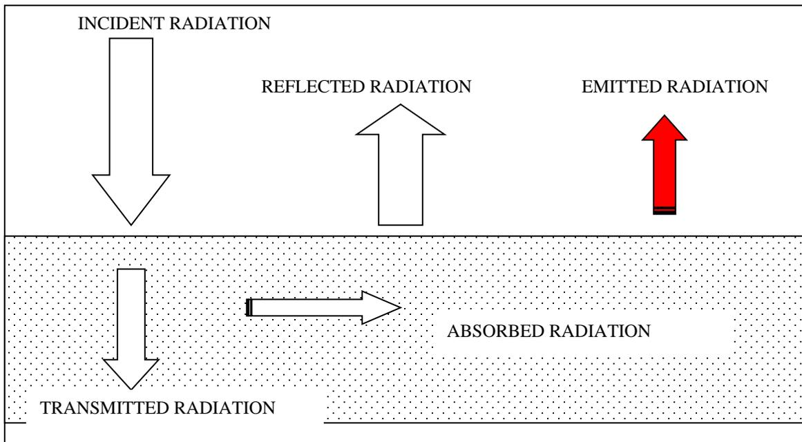
Conservation of energy requires that monochromatic radiation incident upon any surface,  $I_i$ , is either reflected,  $I_r$ , absorbed,  $I_a$ , or transmitted,  $I_t$ . Thus
