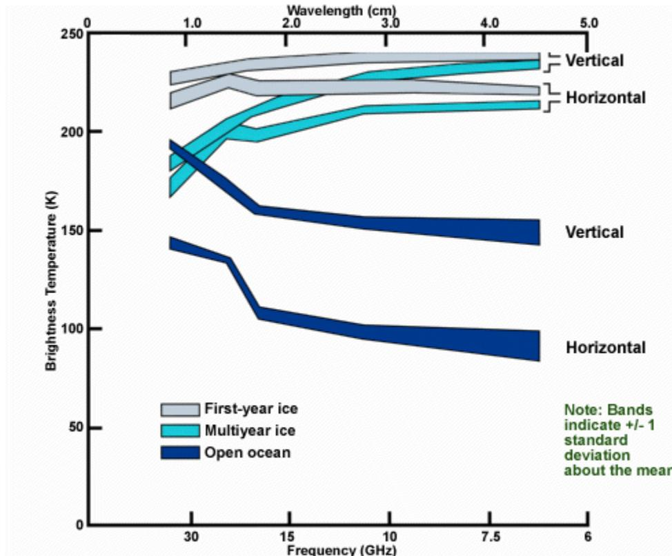
**Figure 3.4** Microwave brightness temperature (at vertical and horizontal polarizations) as a function of frequency (wavelength) of first year sea-ice, multiyear sea-ice, and sea water as observed by the Nimbus-7 SMMR (Scanning Multichannel Microwave Radiometer) (Cavalieri et al. 1984).
