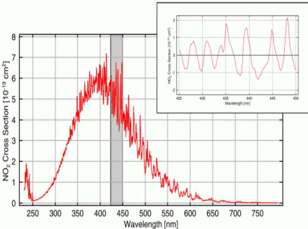
**Figure 10.1** The absorption cross-section of NO<sub>2</sub> in the wavelength range covered by GOME and in the region often used for NO<sub>2</sub> retrieval (inset). The latter is already high pass filtered to highlight the differential structures which are used to separate absorption by trace species and extinction by scattering.
