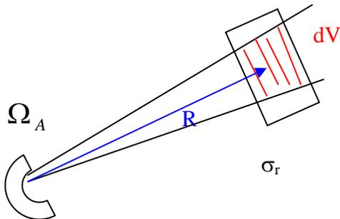
Using the Friis transmission formula, we can find the power intercepted by the object  $P_{\text{int}}$  as
