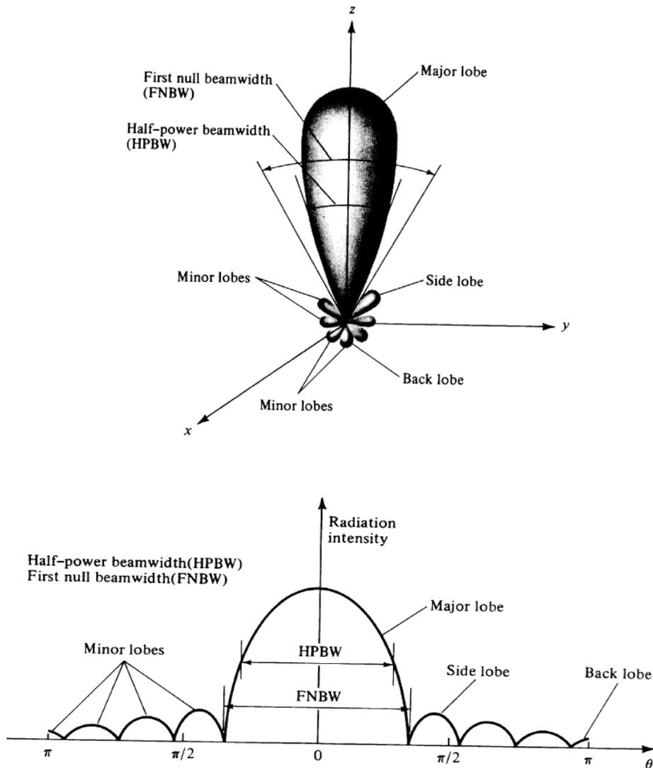
**Figure 14.2** Antenna power pattern in polar coordinates and in rectangular coordinates.
