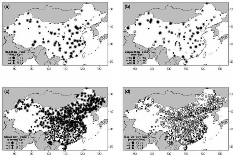
**Figure 1.** Trends in (a) annual mean solar irradiance ( $\text{W/m}^2$  per 10yr) and (b) pan evaporation (mm per 10yr) for 1955–2000. Trends in (c) annual mean total cloud cover (percent per 10yr) and (d) frequency of occurrence of cloud-free sky (percent per 10yr) for 1954–2001. Station trend indicators with circle around them are significant at the 90% confidence level.
