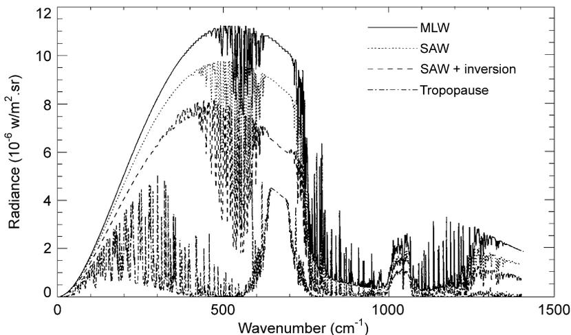
Fig. 1. Downward spectral radiance at the surface level calculated with MODTRAN for an incident angle of  $53^\circ$  and for three different atmospheric temperature profiles: standard mid-latitude winter (MLW), sub-arctic winter (SAW), sub-arctic winter with a  $-20^\circ\text{C}$  surface inversion in the lower kilometre. The last curve represents the radiance at the tropopause level in SAW conditions.
